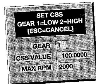
Figure 2-13 Note that the EZPATH has no electronic knowledge about what the spindle gear is; you must tell it here if it is to operate properly and safely.
