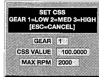
Figure 6-10 When using constant surface speed, make sure that the X=0 position remains the spindle centerline.
